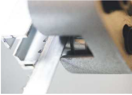
▲ A neat feature is the use of double bearings for blade support
